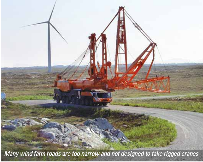
Moving cranes fully or partially rigged can have disastrous results
