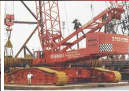
Alf proudly stands next to a new Demag CC4000 crawler crane in Brazil.
