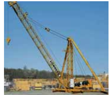
The new 200 DR 5-10 derrick crane for dismantling internal climbing tower cranes from high buildings.
