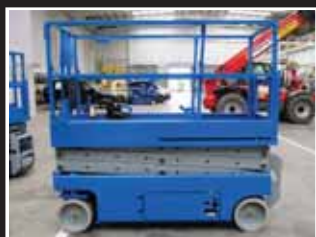
Genie GS-2032 Battery scissor lift 8.10m/363kg - 2005/6
