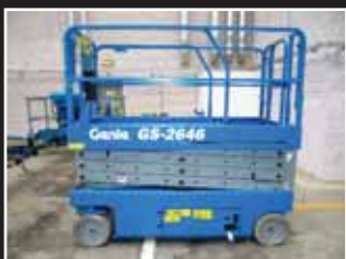
Genie GS-2646 Battery scissor lift 9.92m/454kg - 2005/6/7/8
