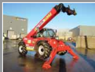
Manitou MT 1840 Telescopic forklift 18m/4 Tonne - 2008
