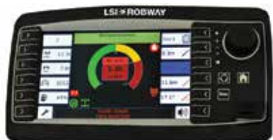
Load Systems' RCI-8510 manages all aspects of the crane and has an extensive load chart memory.
