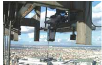
The auto-focus zoom camera means the operator can view the load from directly above
