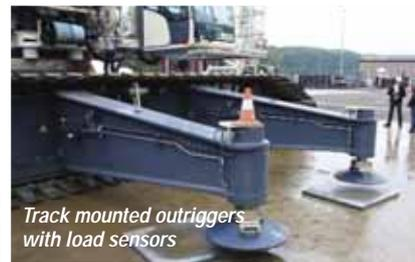
Track mounted outriggers with load sensors
