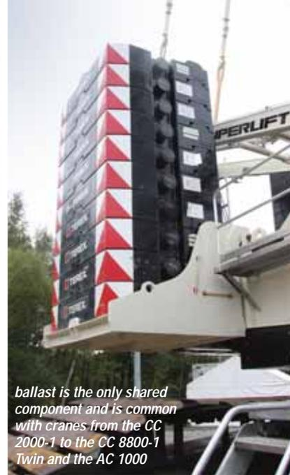
ballast is the only shared component and is common with cranes from the CC 2000-1 to the CC 8800-1 Twin and the AC 1000
