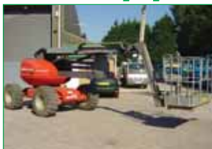
SELF PROPELLED TELESCOPIC PLATFORM 2001 MANITOU 165 16.5m working height (54ft) 4 Wheel Drive, Fly Jib
