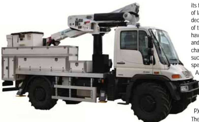
AT36M-Unimog-U400 caption The Altec AT36-M insulated access platform fitted with material handling for the general maintenance of overhead power lines rated to (Category C) 46kV working voltage for working on live lines.
