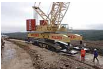
The LR1400/2 was first in the narrow wind farm crawler concept
