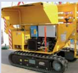
The massive steel plate covers enclose everything for full protection from falling timber and for driving through heavy brush
