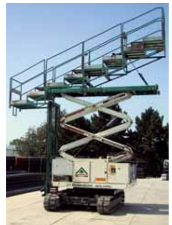
An unusual hydraulic stepped platform for work on sloped ceilings
