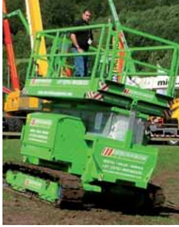
The Holland Lift X105DL22-TR levels by up to six degrees
