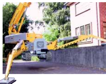
Spider outriggers provide incredible levelling ability
