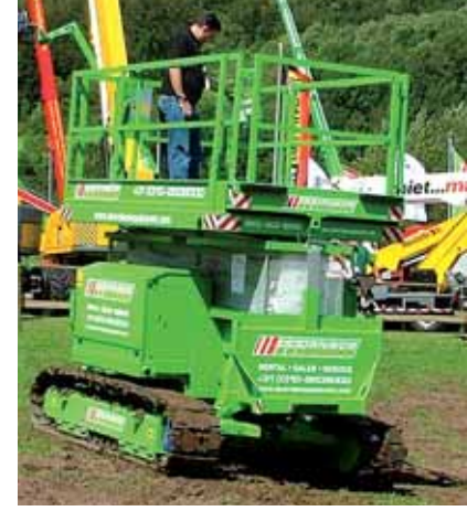
The Holland Lift X105DL22-TR levels by up to six degrees
