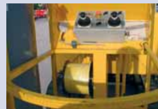
The Custers platform with protected controls, curved rail and tie reel
