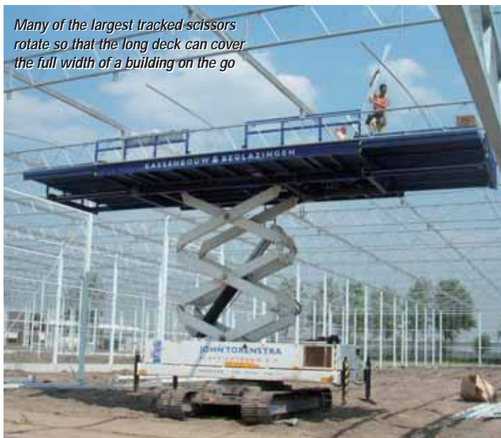
An unusual hydraulic stepped platform for work on sloped ceilings
