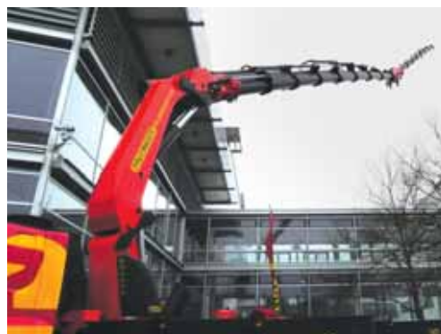
The PK200002 L has a maximum reach of 50 metres.
