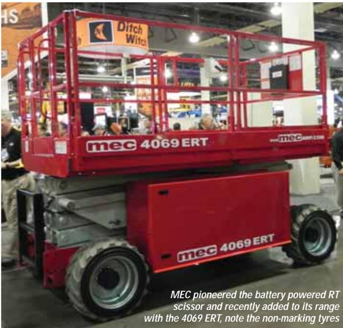
MEC pioneered the battery powered RT scissor and recently added to its range with the 4069 ERT, note the non-marking tyres
