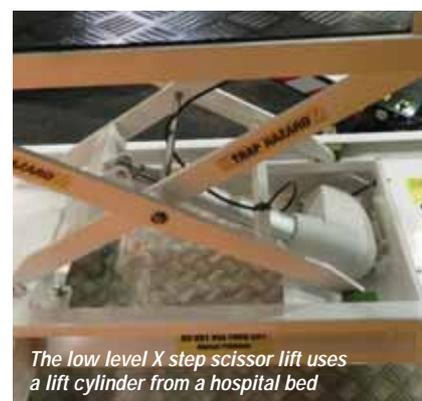
The low level X step scissor lift uses a lift cylinder from a hospital bed
