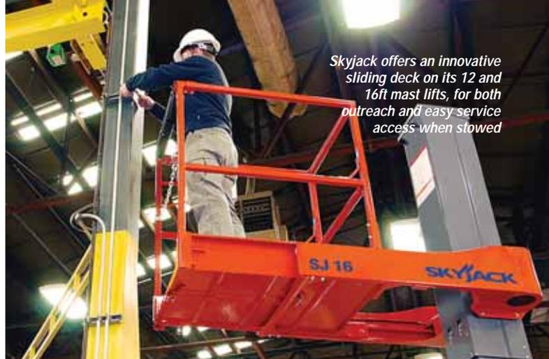
Skyjack offers an innovative sliding deck on its 12 and 16ft mast lifts, for both outreach and easy service access when stowed
