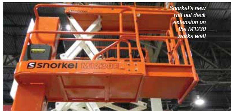
Snorkel's new roll out deck extension on the M1230 works well
