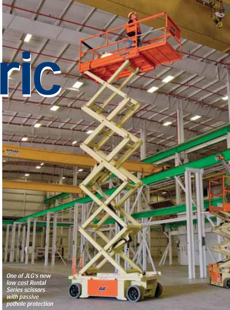
One of JLG's new low cost Rental Series scissors with passive pothole protection
