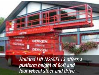
Holland Lift N265EL13 offers a platform height of 86ft and four wheel steer and drive
