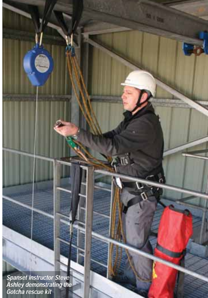
The extendable pole and special 'frog' clip enable the rescuer to carry out the rescue from a point of safety
