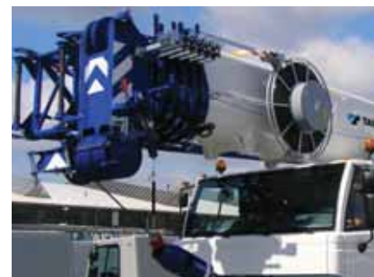
Conductix-Wapfler's double hose reel attached to a Tadano Faun ATF90G-4 All Terrain crane.
