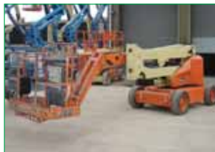
SELF PROPELLED TELESCOPIC 2001 JLG M45J. 15.5m working height (51ft). Fly Jib, Bi-Energy.
