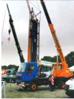
Crowland Cranes showed off this cost effective, refurbished eight tonne capacity Tadano TS75 mounted on a DAF LF 45.150 chassis
