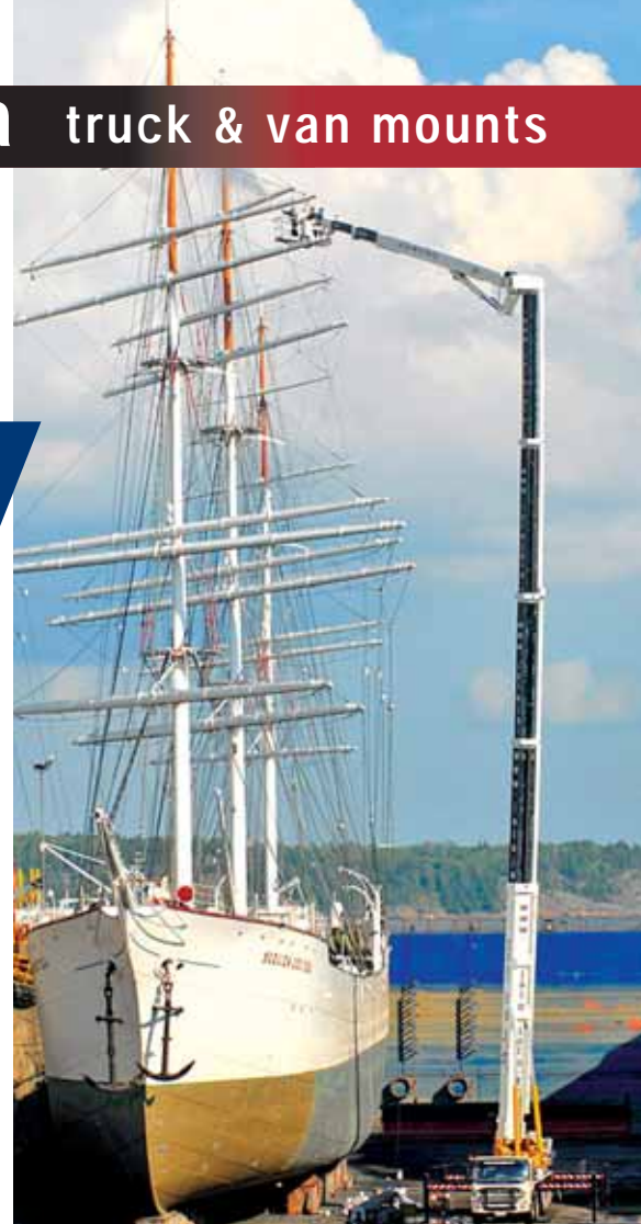
A 90 metre Bronto Skylift S 90 HLA owned by the Finnish contractor Jalo & Jalo was recently used for painting the masts of the full-rigger Suomen Joutsen which was built in France as a freighter in 1902. UK Bronto dealer Blue Line Access says it has interest in a similar sized unit.
