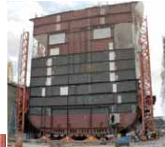
ALE Lastra devised a hydraulic skidding system to insert the new mid-body section
