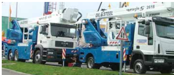
Oil&Steel's latest Eagle truck mounted platforms seen at Intermat - the S2618 on an Iveco Eurocargo chassis and a MAN based S4230
