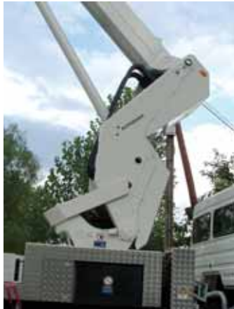
Ruthmann's tilting superstructure frame claims to reduce tailswing and also allows additional levelling
