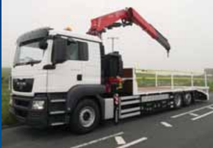
New 6x2 Man 26-400. Fassi F275 remote crane with flat or cheese wedge body.
