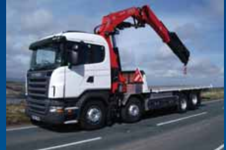
2009 & 2010 8x2 Scania R420. Fassi F660 remote crane with flat or cheese wedge body
