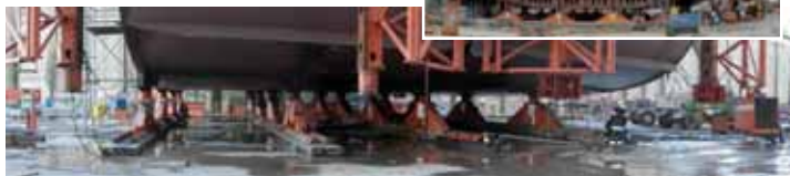
ALE Lastra devised a hydraulic skidding system to insert the new mid-body section
