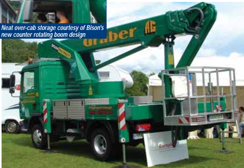
Bison's counter rotating superstructure keeps the overall length of the machine to a minimum
