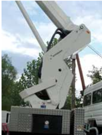
Ruthmann's tilting superstructure frame claims to reduce tailswing and also allows additional levelling
