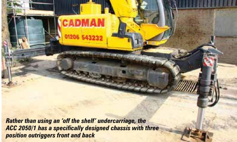
*Rather than using an 'off the shelf' undercarriage, the ACC 2050/1 has a specifically designed chassis with three position outriggers front and back*
