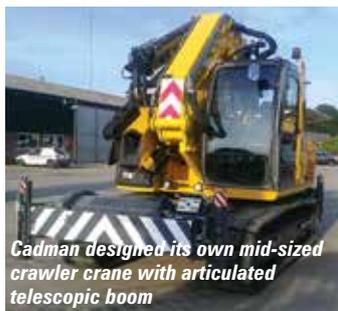
*Cadman designed its own mid-sized crawler crane with articulated telescopic boom*
