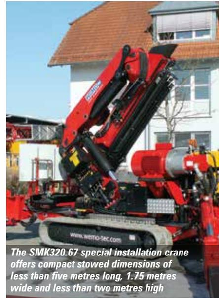
The SMK320.67 special installation crane offers compact stowed dimensions of less than five metres long, 1.75 metres wide and less than two metres high
