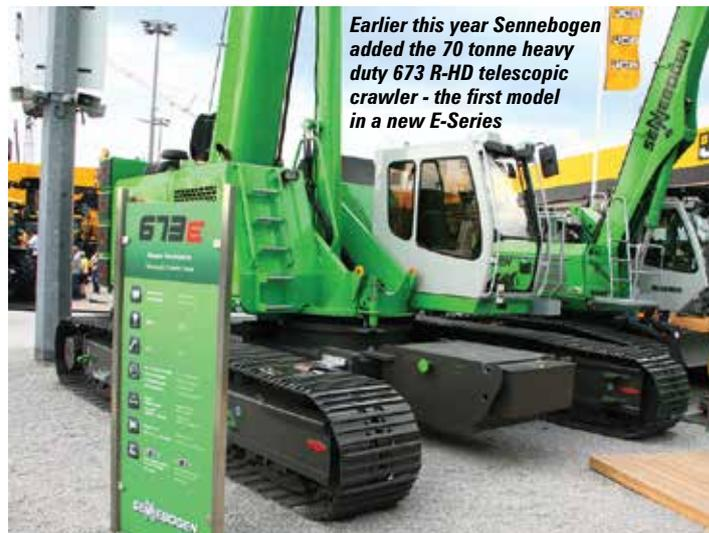
Earlier this year Sennebogen added the 70 tonne heavy duty 673 R-HD telescopic crawler - the first model in a new E-Series
