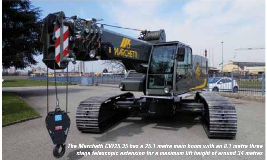
*The Marchetti CW25.35 has a 25.1 metre main boom with an 8.1 metre three stage telescopic extension for a maximum lift height of around 34 metres*
