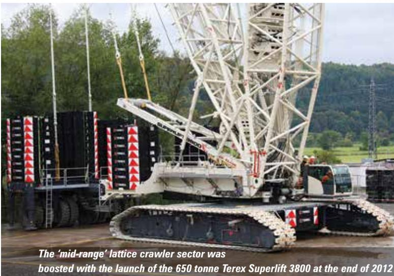
The 'mid-range' lattice crawler sector was boosted with the launch of the 650 tonne Terex Superlift 3800 at the end of 2012
