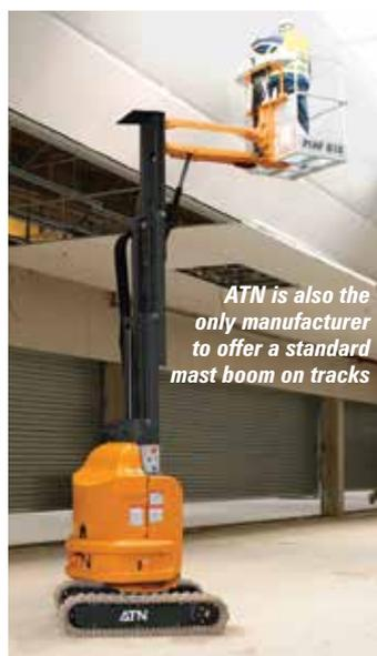
ATN is also the only manufacturer to offer a standard mast boom on tracks
