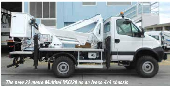
The new 22 metre Multitel MX220 on an Iveco 4x4 chassis
