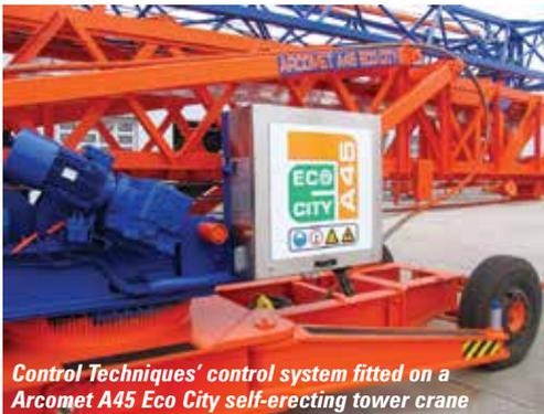
Control Techniques' control system fitted on a Arcomet A45 Eco City self-erecting tower crane
