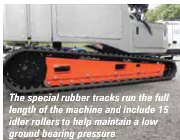
*The special rubber tracks run the full length of the machine and include 15 idler rollers to help maintain a low ground bearing pressure*
