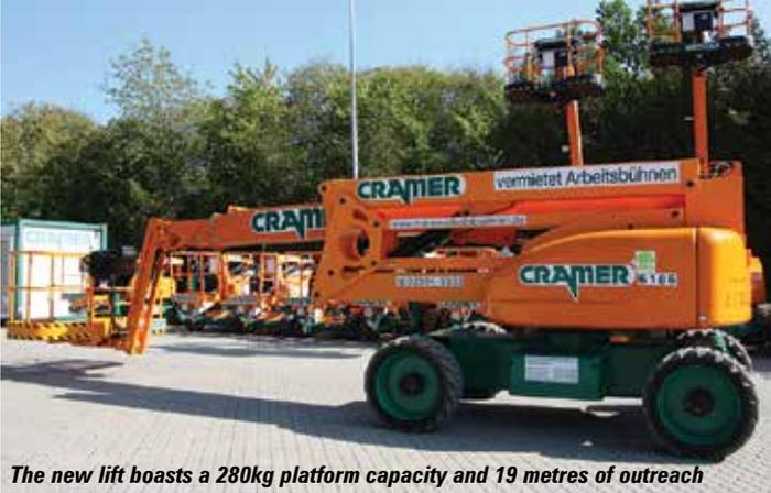
The new lift boasts a 280kg platform capacity and 19 metres of outreach
