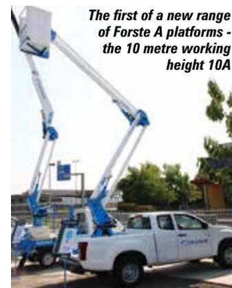
*The first of a new range of Forste A platforms - the 10 metre working height 10A*
