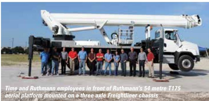
*Time and Ruthmann employees in front of Ruthmann's 54 metre T175 aerial platform mounted on a three axle Freightliner chassis*
