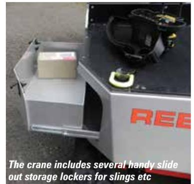
*The crane includes several handy slide out storage lockers for slings etc*
