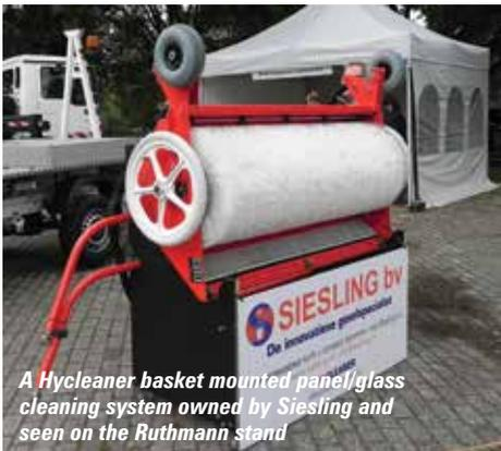
A Hycleaner basket mounted panel/glass cleaning system owned by Siesling and seen on the Ruthmann stand
