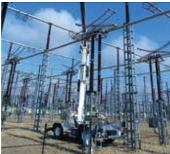
French aerial work platform manufacturer France-Elévateur has launched a new 17 metre articulated boom lift - the 172 ATBI - for live line work.
