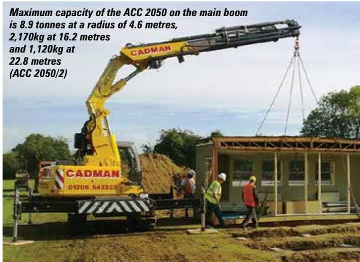
*Maximum capacity of the ACC 2050 on the main boom is 8.9 tonnes at a radius of 4.6 metres, 2,170kg at 16.2 metres and 1,120kg at 22.8 metres (ACC 2050/2)*
