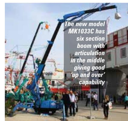
**The new model MK1033C has six section boom with articulation in the middle giving good 'up and over' capability**
