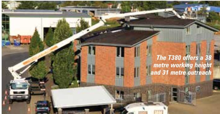
*The T380 offers a 38 metre working height and 31 metre outreach*
