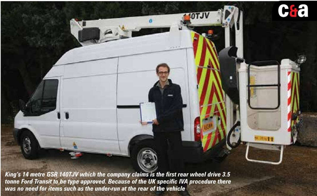
*King's 14 metre GSR 140TJV which the company claims is the first rear wheel drive 3.5 tonne Ford Transit to be type approved. Because of the UK specific IVA procedure there was no need for items such as the under-run at the rear of the vehicle*
