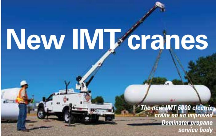
The new IMT 6000 electric crane on an improved Dominator propane service body
