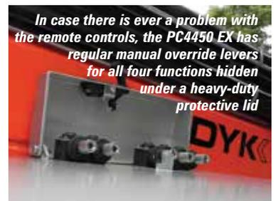
*In case there is ever a problem with the remote controls, the PC4450 EX has regular manual override levers for all four functions hidden under a heavy-duty protective lid*
