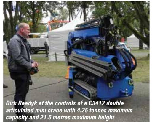
Dirk Reedyk at the controls of a C3412 double articulated mini crane with 4.25 tonnes maximum capacity and 21.5 metres maximum height
