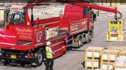
The new cranes have been fitted with Hiab's Operator Protector System and can be operated either with the remote controller or from a raised standing platform fitted to the crane. The company said its drivers particularly like the ease-of-use, responsiveness and precision of the radio remote controls.
