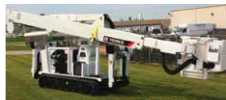
The unit is 990mm wide but expands to 1.3 metres for greater stability.
