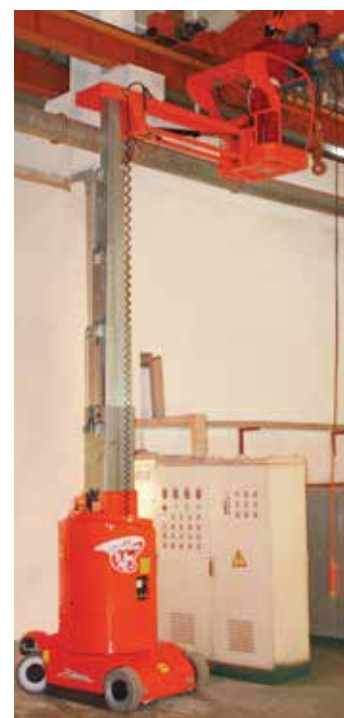
Dingli's first mast boom has an 11.5 metre working height
