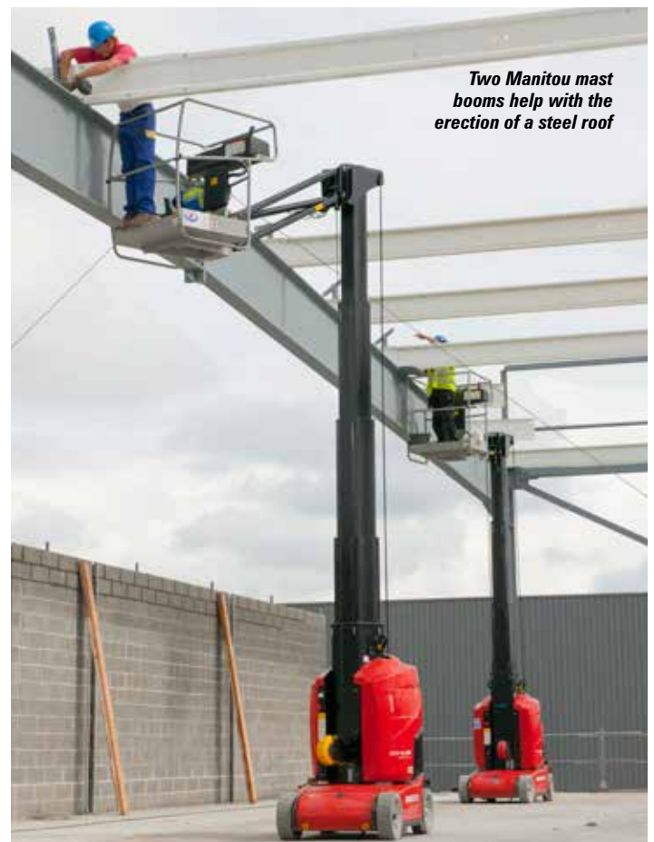
Genie has two models - the GR20J and the GR26J - built by Manitou and based on its eight and 10 metre VJR models
