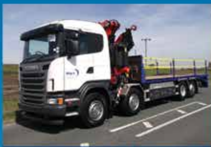
New Scania 8x2 G400. Fassi 455 remote crane with cheese wedge body
