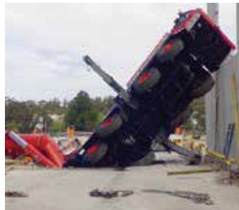
This 250 tonne crane found the one missing deck support prop among hundreds.
