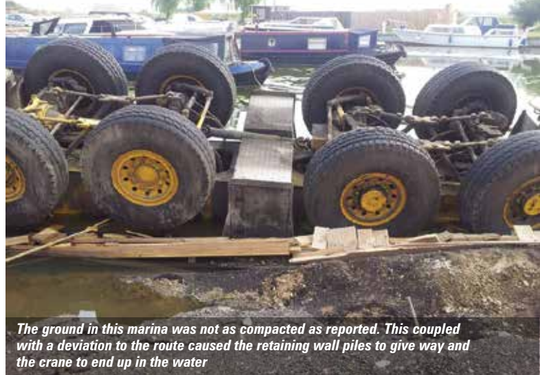
Setting up on the edge of an excavation requires a great deal of accurate information and planning. If possible it should be avoided
