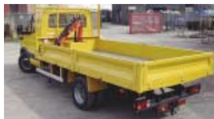
Spenborough Engineering is now using the stronger and lighter ultra high yield steel in its new range of bodies
