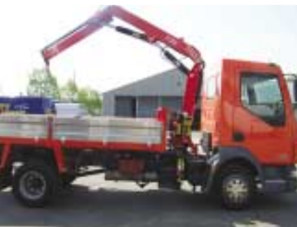
Suited to 7.5 GVW vehicles the F50A.21 weighs 605kg and has a maximum radius of 4.9 metres and a 960kg lift.
