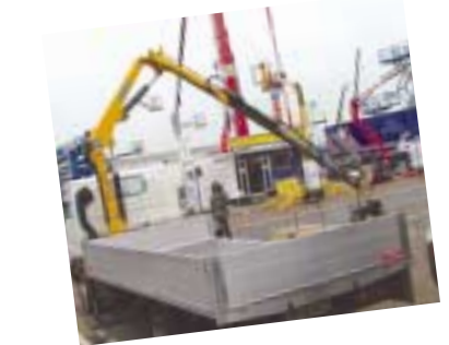
Effer showed its Easy power 30 for a 3.5 tonne truck with 7.8m outreach
