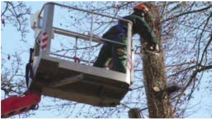
Teupen's rotating platform provides handy outreach when taking a tree down piece by piece.
