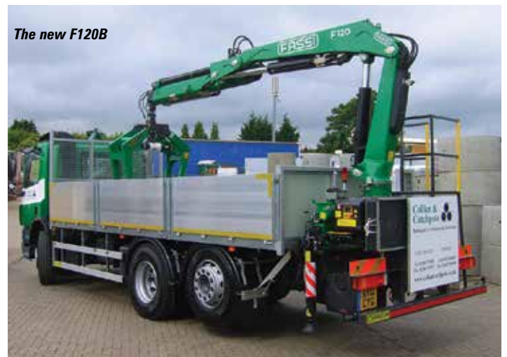
Maximum reach for the new crane is around 50 metres with the jib able to articulate above horizontal
