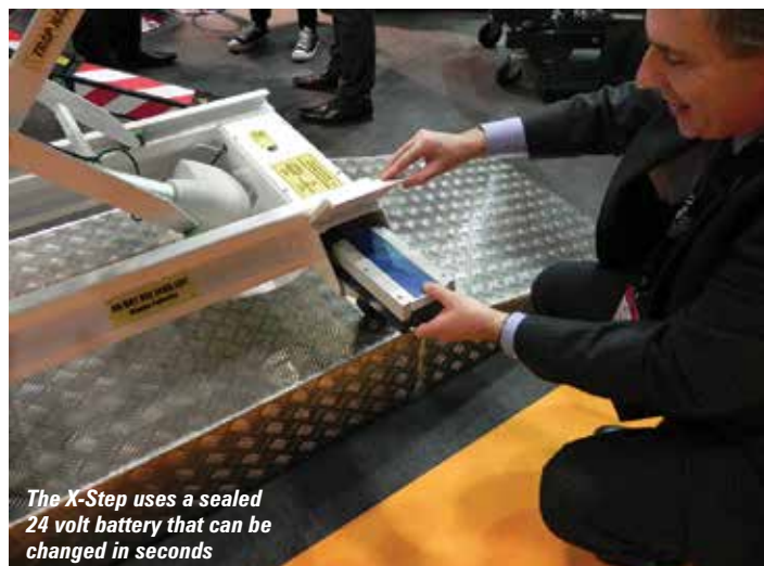
Hinowa has pioneered lithium battery power options on spider lifts
