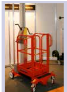
The Access Platform Company's launched its new 4.5 metre Skywinder Mini 250 which makes use of an additional mast section to offer an extra metre working height compared to the original Skywinder Mini. Slightly heavier at 280kg the 250 offers a 136kg platform capacity
