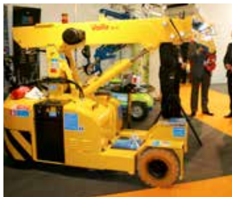
Hird showed a 2.5 tonne Valla 25EL pick&carry crane and a Winlet 350 glazing robot.
