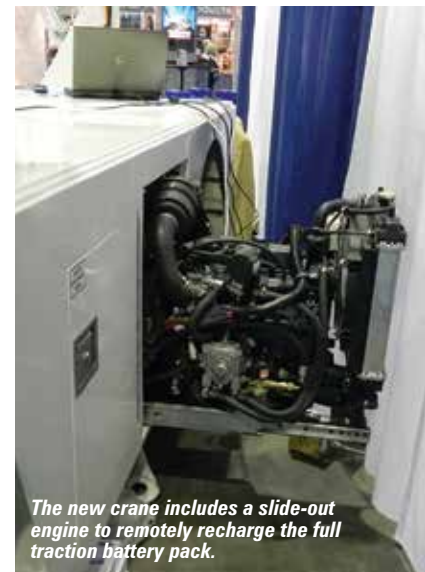
The newly formed Bailey Crane showed a new 8 tonne hybrid carry deck crane.
