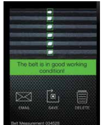
Determining belt wear.
