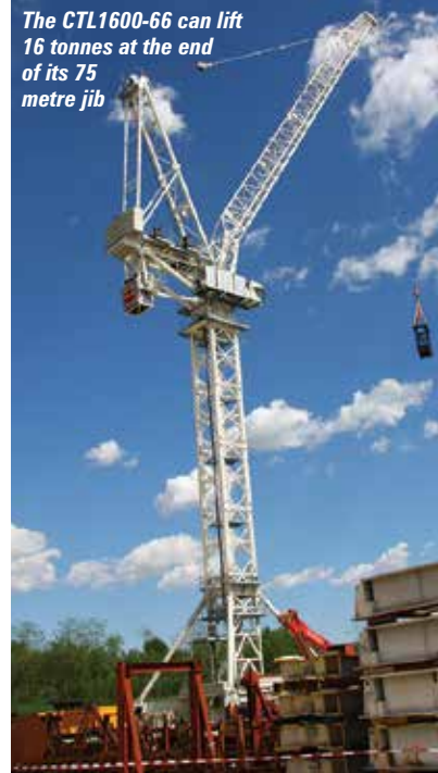
The new HD33 tower system uses six metre by 3.3 metre sections
