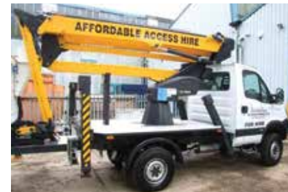
The new 26 metre articulated Co.Me.t Eurosky 26 truck mounted lift
