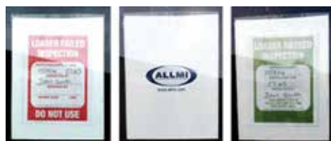
The completed check sheet is slipped into a windscreen mounted display holder
