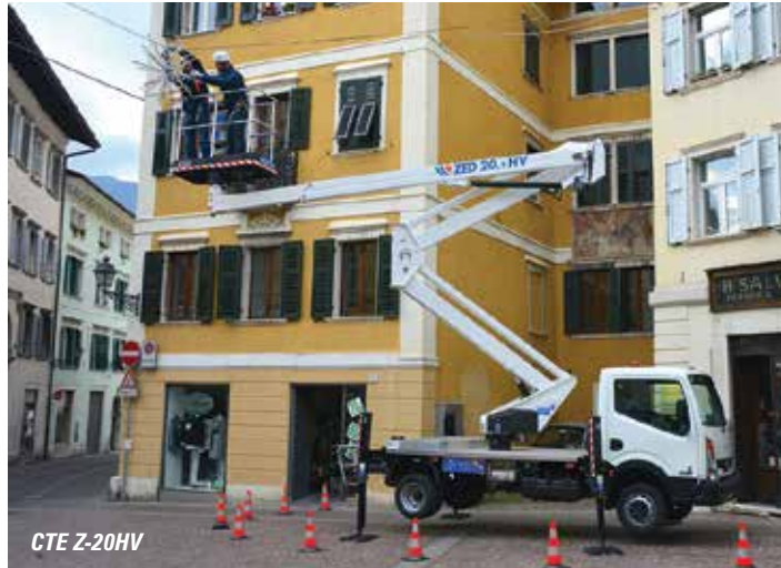
Co.Me.T's new insulated van mount has no internal pillar
