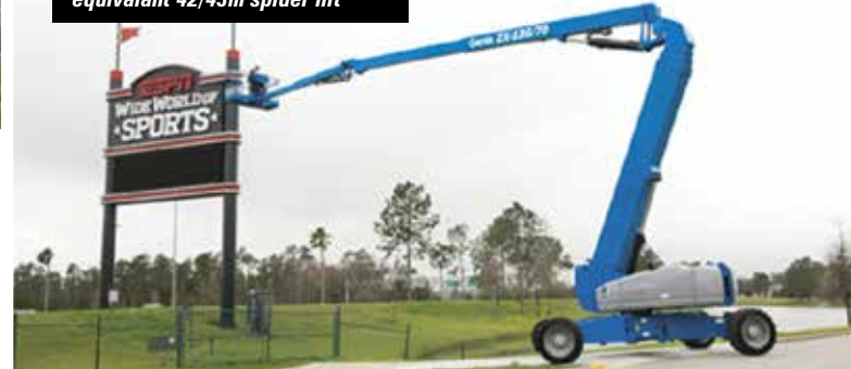
A JLG 1350SJP (above) and Genie ZX135/70 (below) are physically much bigger and heavier than the equivalent 42/43m spider lift
