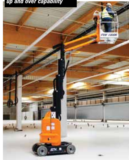
Mast booms have a useful up and over capability
