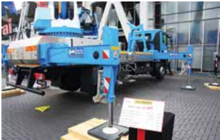
The new 48 metre, 31.5 metre outreach, two axle Palfinger P480.
