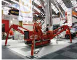
Easy Lift showed its new 36 metre R360 lithium hybrid tracked spider alongside a lighter weight EV150 van mount. Look out for a 41 metre spider at the end of the year.
