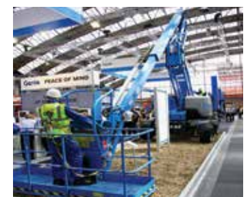
Second new articulated boom from Genie was the 60ft Z-62/40 with 12.42 metres of outreach.
