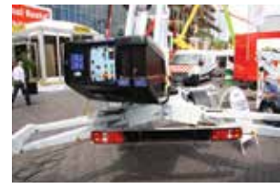
Dinolift had its updated version of its 180XT II with spider type outriggers for better levelling and outreach.
