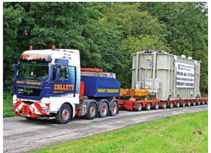
Collett delivered two 200 tonne transformers using its girder bridge trailer. Here a 14 axle modular flat top trailer moves one transformer to its holding location
