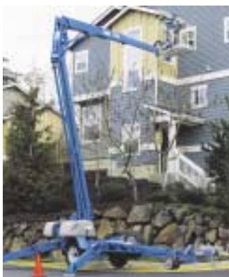
Articulating-telescopic machines like this Genie are great when you need to get up and over
