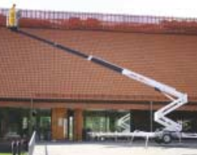
The Dino 260XT features a sigma riser
