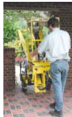
The retractable axle on Nifty's 90 allows it to fit through a single personnel door
