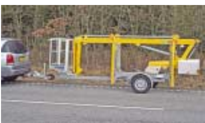
Trailer lifts are easy to move over long distances without specialist vehicles.
