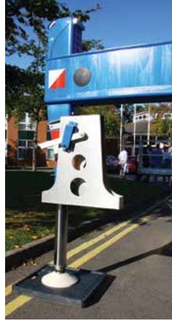
Palfinger's P480 - stores each outrigger pad at the end of the outrigger.
