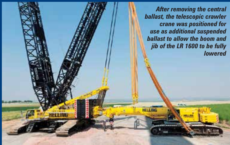
The LR 1600/2s boom being re-installed by the LTR 1220
