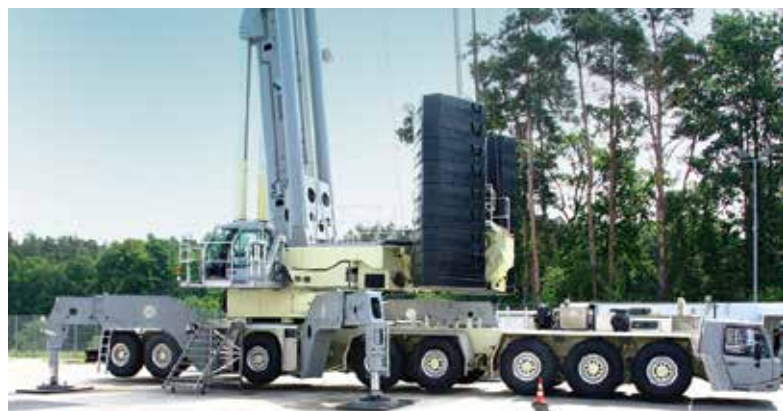
At just under 20.5 metres the Tadano has a long chassis but has a good turning circle, large counterweight, competitive road speed and compact outrigger spread
