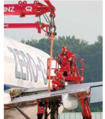
Sophisticated hanging gear: the combination of cross and spreader beams was able to adjust the angle to the appropriate centre of gravity using an electric chain hoist.
