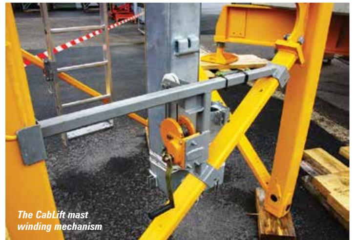
The CabLift mast winding mechanism
