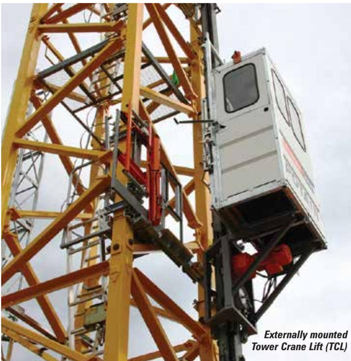
Externally mounted Tower Crane Lift (TCL)
