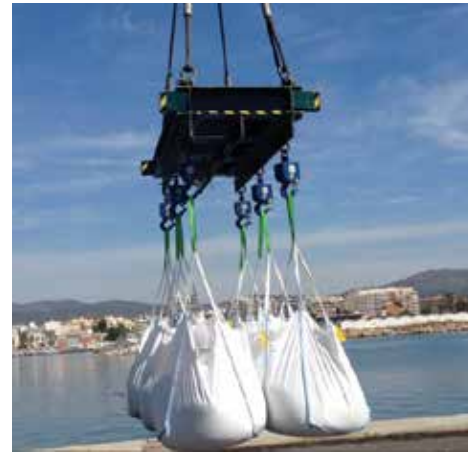
Elebia's latest hooks now feature integrated load cells and the new eMax control system.
