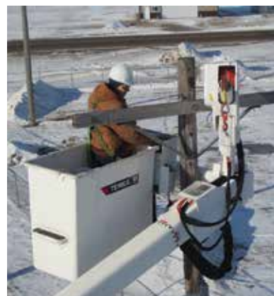
The swing arm combined with the 180 degrees of platform rotation allows an operator to cover both sides of a pole from a single position.
