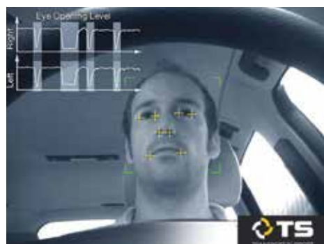
Transport Support's warning system monitors whether a driver is drowsy or inattentive.
