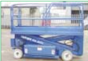
SELF PROPELLED SCISSOR 1999 UpRight SL20 8m Working Height (26ft) Non-marking tyres, Dual voltage charger.
