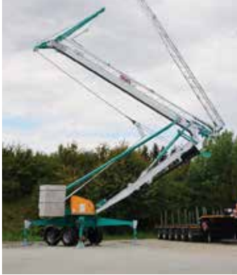
Cattaneo's new 2.2 tonne CM 271 self-erecting tower crane
