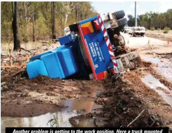
Another problem is getting to the work position. Here a truck mounted platform and crawler crane find that the edge of the road was not as stable as initially thought
