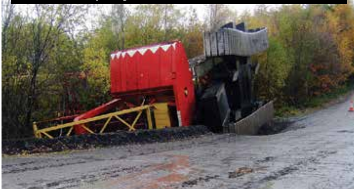
Another problem is getting to the work position. Here a truck mounted platform and crawler crane find that the edge of the road was not as stable as initially thought
