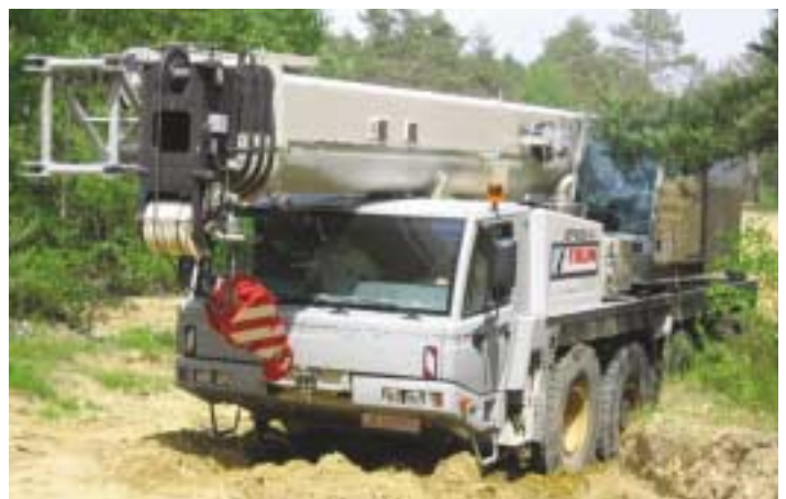
Tadano Faun's new ATF 65G-4 features the Faun all wheel steering system for improved rough terrain capability
