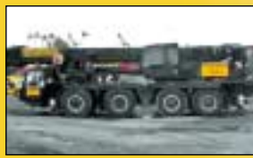
Faun ATF70-4 Year 1995/8. Capacity 70 tonnes. All terrain
