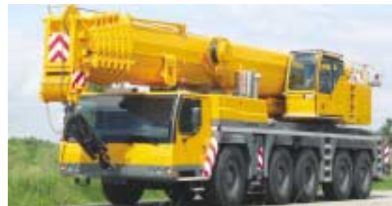
The Liebherr LTM 1200-5.1 has a 72 metre main boom and so offers a long-boom alternative to the stronger LTM 1220-5.1, which has a 60 metre boom.
