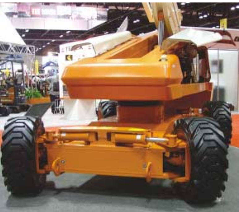
The new Snorkel TB85J has fixed axles and over 23 metres outreach.
