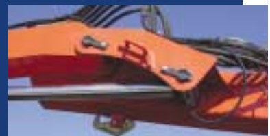
Linkages and pins between booms
